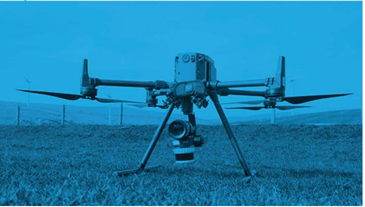
Clobotics IBIS<sup>™</sup> platform is built on a DJI Matrice 300 RTK drone, with a customized data acquisition system including high-resolution cameras, intelligent sensors, and powerful onboard computing. It has been specifically developed for wind turbine inspections and designed to ensure cost-effective operations and economies of scale in the hardware system.
