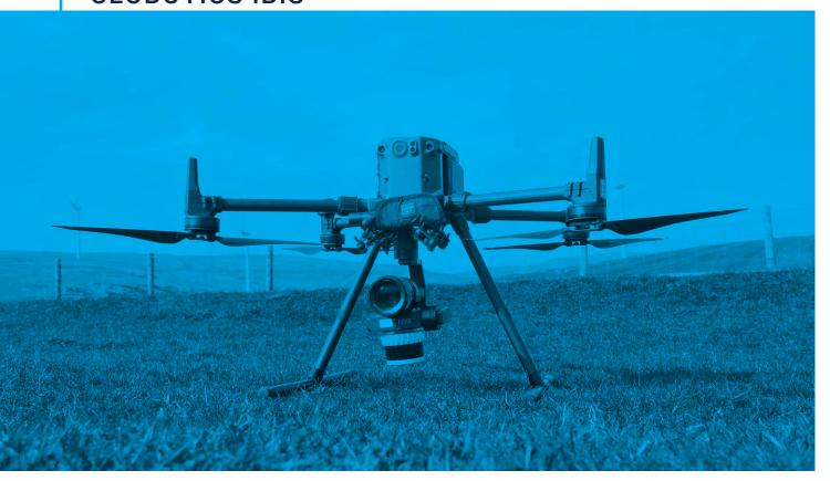
Clobotics IBIS™ platform is built on a DJI Matrice 300 RTK drone, with a customized data acquisition system including high-resolution cameras, intelligent sensors, and powerful onboard computing. It has been specifically developed for wind turbine inspections and designed to ensure cost-effective operations and economies of scale in the hardware system.
